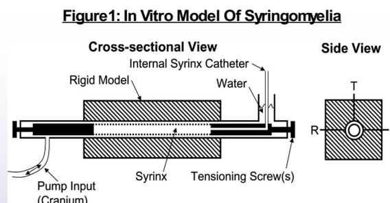
To make sure the model accurately represented the human body, the entire apparatus was placed into the same MRI which was used on the volunteer and the CSF velocity was matched accordingly.
